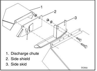
Figure 15. Side Skids, Side Shield & Discharge Chute Installation
